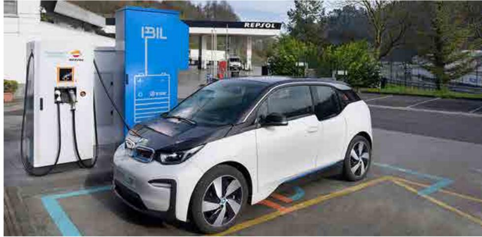
The charging station for electric vehicles that uses energy storage based in recycled batteries from Irizar e-mobility entered into operation in 2021. This charging point for electric vehicles is the first one that uses energy storage based in second life batteries and it has been developed by **Repsol and Ibil**. The charging point was installed in a Repsol service station on the N-I road where it goes through the city of Tolosa in Gipuzkoa.
