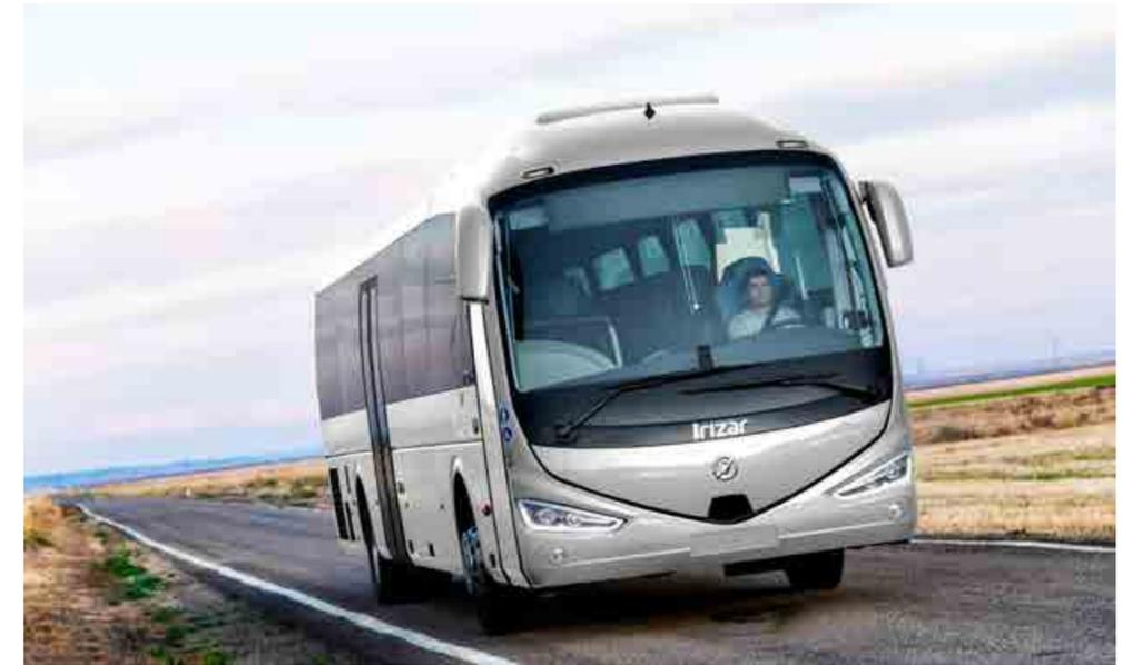
The new generation Irizar i4 coach now offers significant new features that mainly focus on a major reduction in weight and optimal per axle load distribution. The result is a **lightened** vehicle with a weight reduction of up to 955 kg, depending on the configuration chosen.
